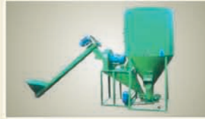
Feed Plant (Feed Mixer & Grinder)
