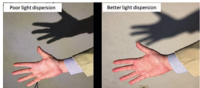
Figure 17. Some LED light sources produce light that is directional, creating sharp shadows which may attract unwanted nesting. Select light sources that produces diffuse light to reduce these shadows.
