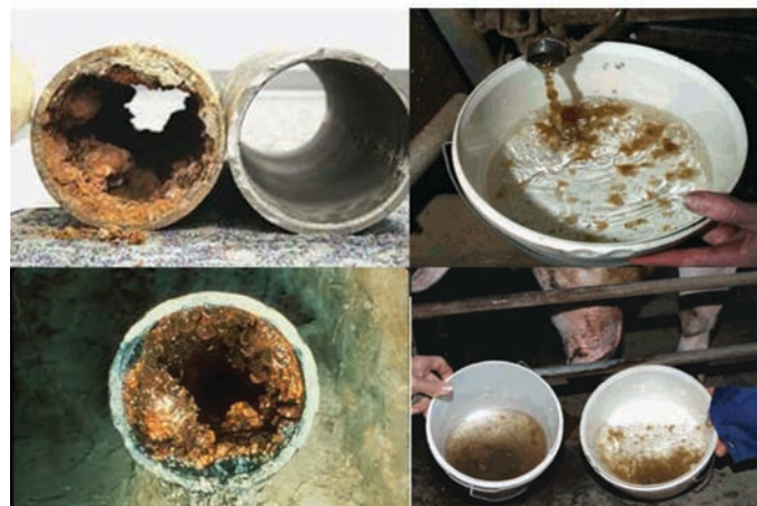
Fig. 3: Biofilms clogging the pipeline
