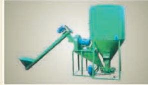
Feed Plant (Feed Mixer & Grinder)
