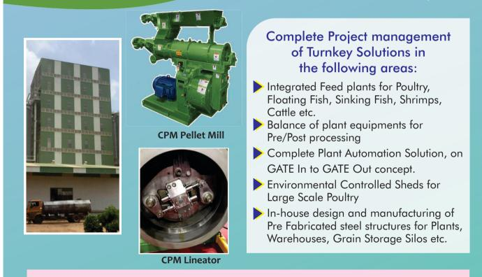
CPM Lineator Technology: Remotely Control the distance between roll and die surface, even when the pellet mill is on. This technology provides swift, accurate and safe roll adjustment, with no downtime, so no production loss.
