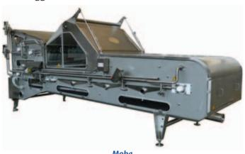
These days, no one should have to sit for hours breaking and separating eggs, which is why Moba has developed the Pelbo Synchro egg breaker and separators. These are high-capacity machines with extremely high yields and, says Moba, proven reliability. Synchro breakers are available in five models with capacities ranging from 20,000 eggs per hour to 226,000 eggs per hour.
