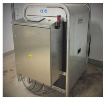
Data about moisture levels are analysed using microwave sensors, and the MMS immediately adjusts the amount of hydrated solution when moisture falls outside of optimal thresholds. Photo: Trouw Nutrition
