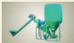
Feed Plant (Feed Mixer & Grinder)
