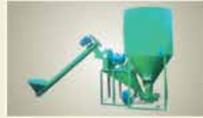
Feed Plant (Feed Mixer & Grinder)
