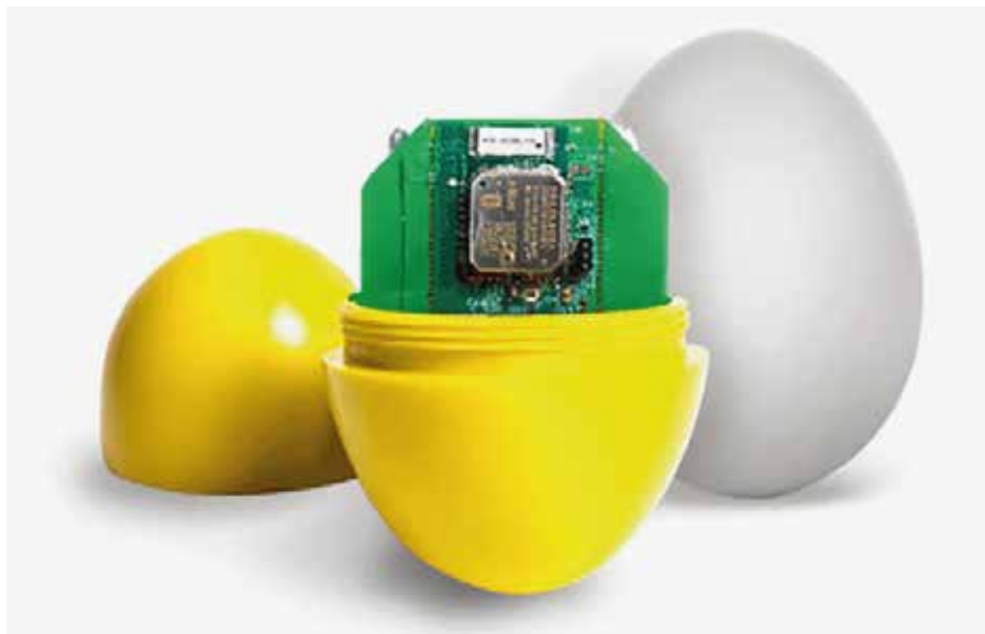
Figure 2: An artificial egg with a G-force sensor inside ( cracklessegg.com )
